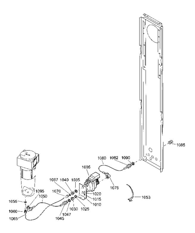
Drain system - Electronic drain system
