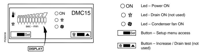
The DMC15 displays DewPoint temperature and controls the condenser fan activation.
