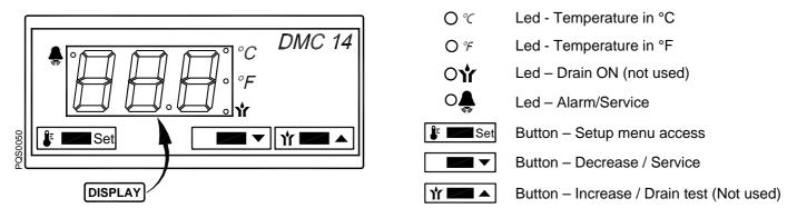
The DMC14 controls the alarms and the settings of the dryer operations.
