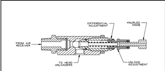
**110998 Series Pilot Valve** (dual control operation)
