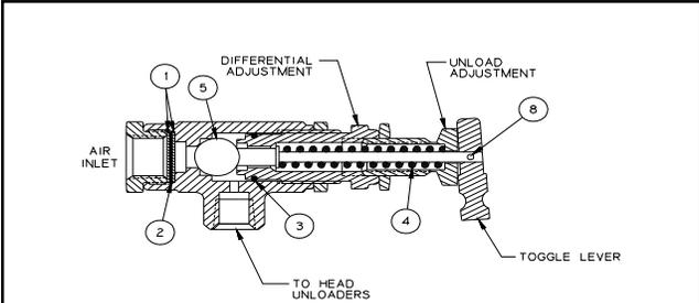
**110832 Series Pilot Valve** (continuous run operation)
